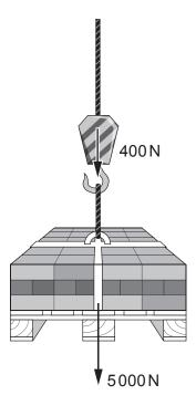
(i) The cable supports the pulley block and bricks. Write down the value of the upward force applied in the cable. [2]
