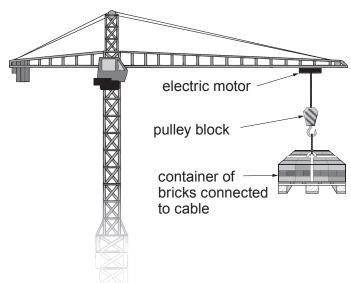
(a) The electric motor is supplied with a voltage of 120 V and a current of 5.0 A to lift the bricks. Use the equation:
